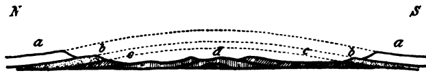
Fig. 106.—Section of the Weald of Kent. a and a , Upper Cretaceous strata, Chalk, forming the North and South Downs; b and b , escarpment of Lower Greensand, with a valley between it and the Chalk; c and c , Weald Clay, forming plains; d , hills formed of Hastings Sand and Clay. The Chalk, etc., once spread across the country, as shown in the dotted lines.
